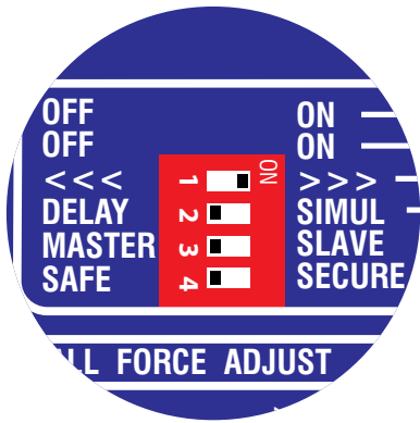
Master DIP Switch Settings
